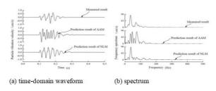
Fig. 8. Comparison between prediction and measured results of the four-hole blastingtest (37#,38#,41#,42#) in the vertical direction of the measuring point 6#
