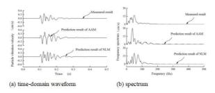
Fig. 6. Comparison between the predicted and measured results of the two-hole blasting test (11#, 12#) in the vertical direction of the measuring point 6#
