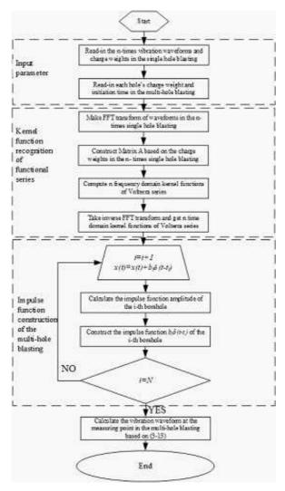
Fig. 2. Flow chart of Volterra functional series model program
